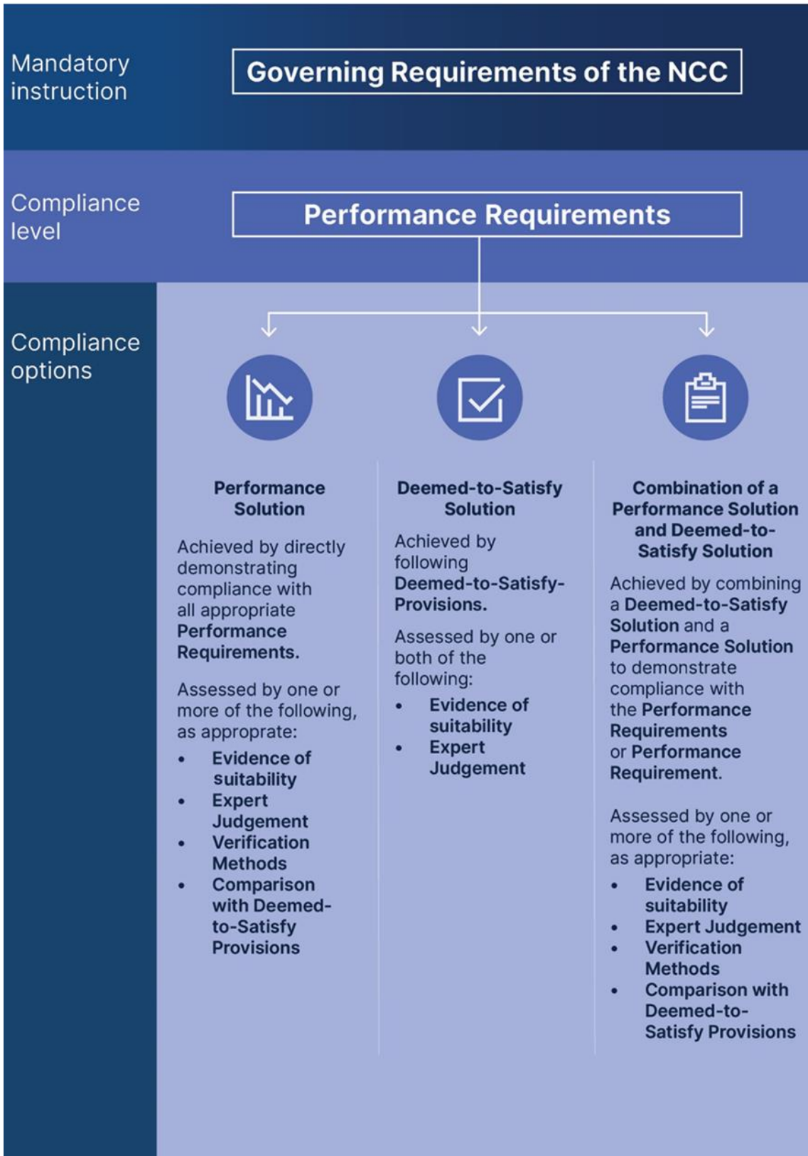
Figure C.1 Demonstrating compliance with the NCC
