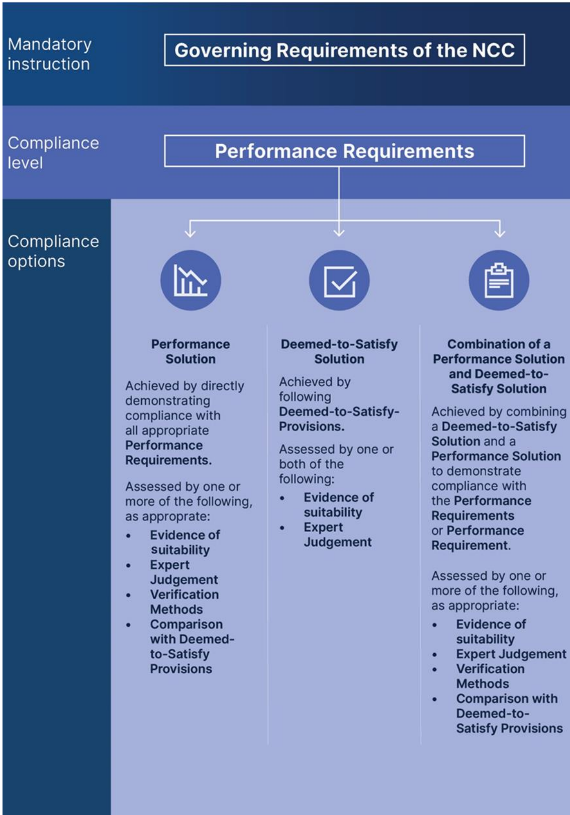
Figure C.1 Demonstrating compliance with the NCC
